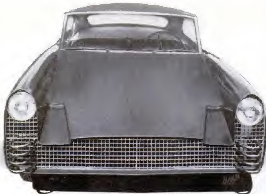
Built by Jay Everett of Los Angeles, a trim sports coupe features an aluminum body and a Cadillac engine
